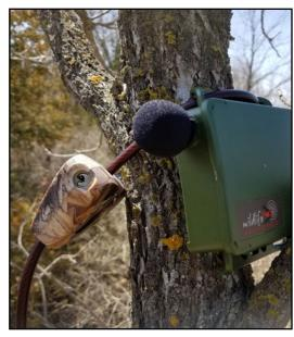
Song meter deployed with locking cable
